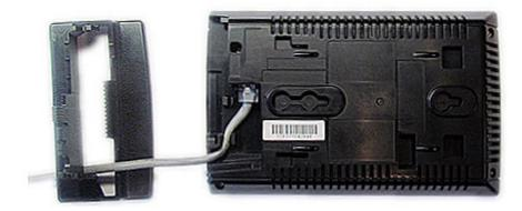
• With the Ethernet cable connected, snap the base attachment into the bottom of the base station and route the cable through the slot in the stand.
